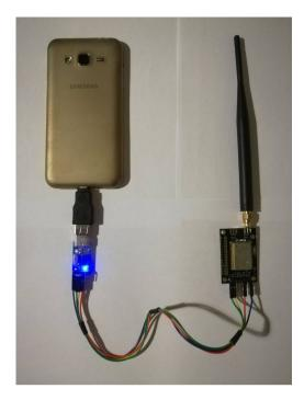
The first one is the module RN2483 which can emit but more importantly, can receive data sent through Lora. These data are transmitted to the USB port of the phone, thanks to an adapter. The phone can also use this port to ask the modem to send a message. The messages are sent Broadcast.
