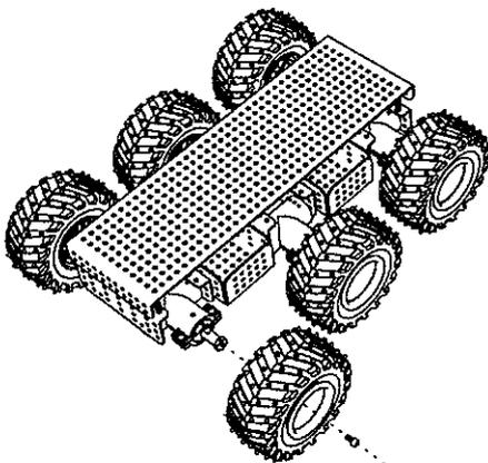
When installing the wheels, the tire profile lines must point at the same direction.
