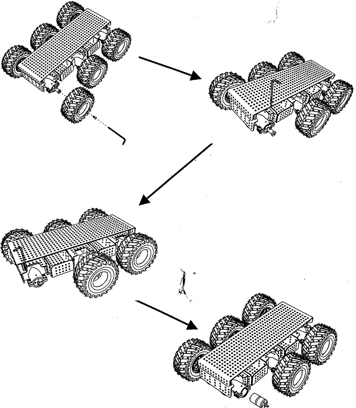
**Adjustment of spring tension**
