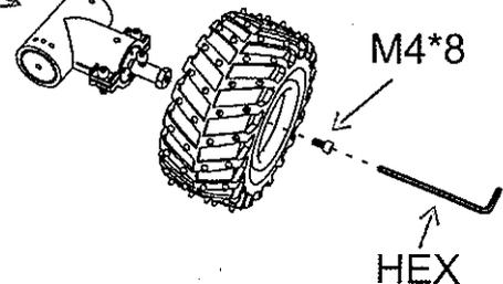
**Replacing the motor
