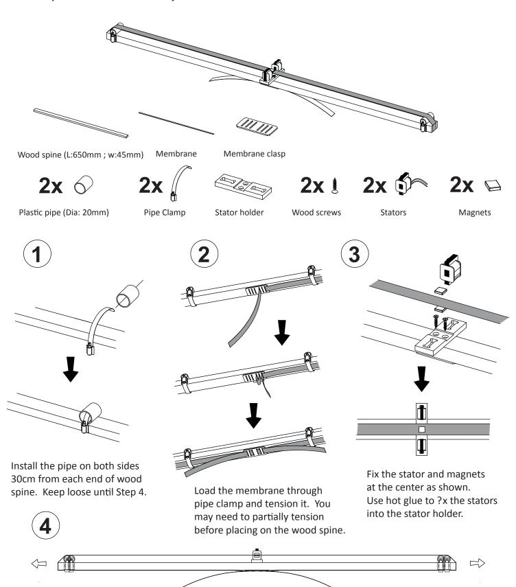
Finally, adjust the pipe position to optimize the output, and then tighten pipe clamps. You can also apply additional tension by placing blocks of wood between the wood spine and the membrane clasp. Note: The membrane should torsionally vibrate at around 20-50 Hz.
