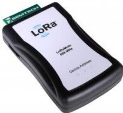
This device was flashed so it can send regularly many information such as the position, altitude, battery level, pressure, temperature, etc... Here, we are mostly interested by the position and altitude. The messages are also crypted so we are the only ones that can read them.
