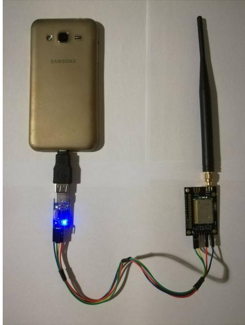
The first one is the module RN2483 which can emit but more importantly, can receive data sent through LoRa. These data are transmitted to the USB port of the phone, thanks to an adapter. The phone can also use this port to ask the modem to send a message. The messages are sent Broadcast. When a message is received, the app analyse it.
