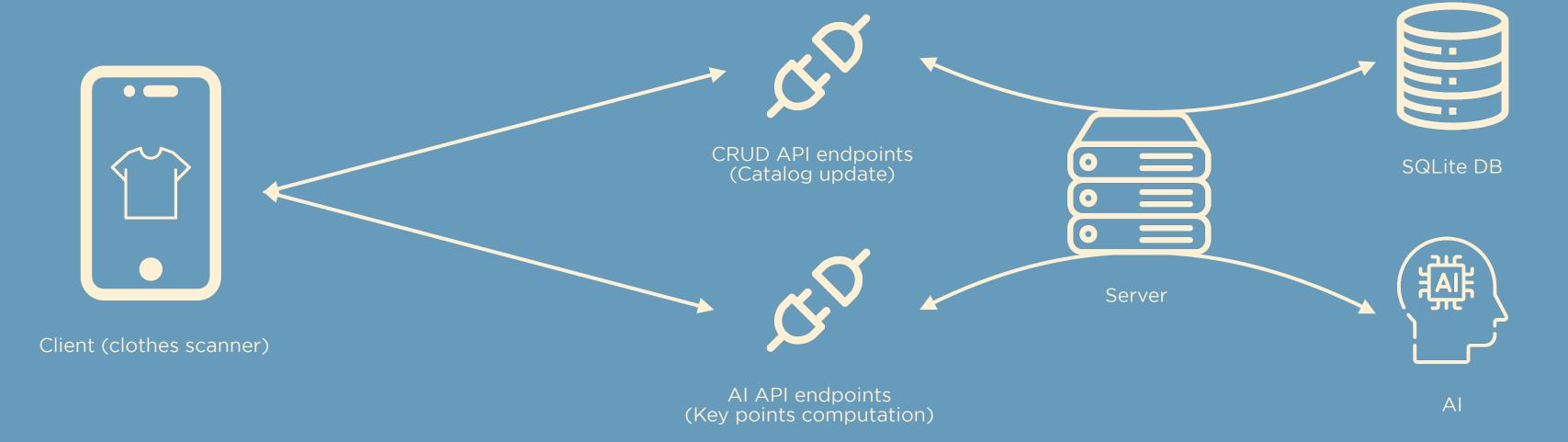
The client communicates with the **AI endpoint** to compute **key point coordinates** on a clothing picture to compute its **dimensions**.
