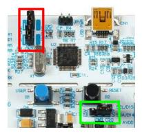
Plug the Nucleo board to your computer with a USB/MiniUSB cable. It automatically opens the folder of the device. (If not, you can find it in /media/\$USER/ on Linux). Just copy your binary file into it and it will flash the Nucleo with it.
