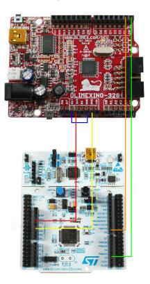
At this point if you power the Olimexino with the USB connection to your computer, the Nucleo will behave normally (executing its program). Now you want to enter Nucleo's bootloader mode :
