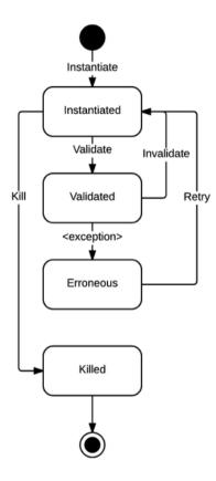
A component's lifecycle defines four states, and is handled by an instance manager that injects runtime dependencies. Many existing python frameworks allow the development and deployment of component-base applications. However, they do not take into account the dynamic aspect of components. The iPOPO component model supports Remote Services, which makes it easy to build distributed applications.
